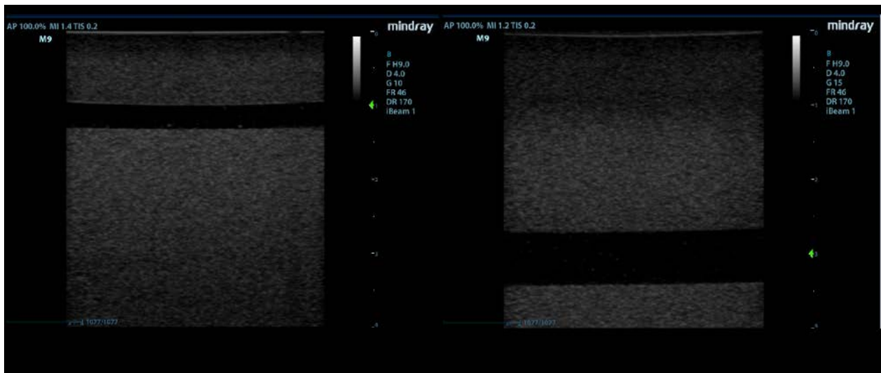
Figure 10. Phantom images showing the near (left) and far field (right) gray scale calibration
