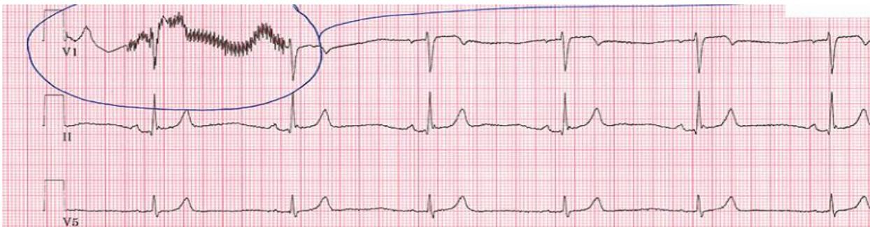
**Figure (10) Wavy V1 baseline due to loose electrode**
